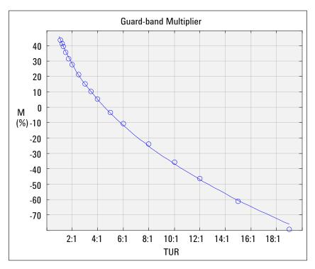
Figure 4 shows M versus TUR from Table 2 using 'o' symbols. The continuous line represents the fitted data using Equation 4 displayed as percentage.
